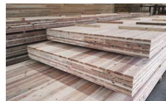
Cross laminated timber is a wood panel product made from gluing layers of solid-sawn lumber together.
